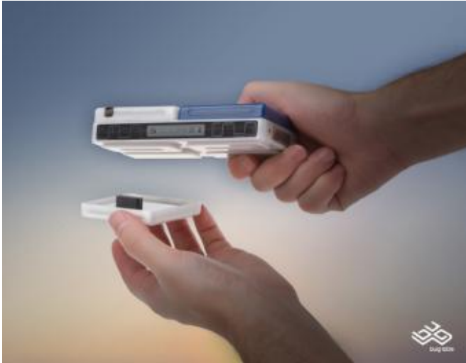
The BUGbase, the hub that every BUGmodule snaps into. Image credit: Bug Labs.
