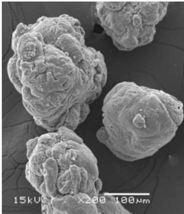
Submicroscopic particles of PVC (shown via electron microscope) and other plastics may pose a previously unrecognized pollution threat. Credit: Courtesy of Emma Teuten, University of Plymouth, UK
