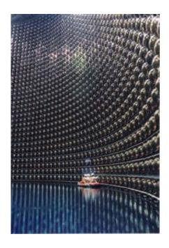
Workers repair one of the 11,200 photomultiplier tubes that line the Super Kamiokande neutrino detector and track the light generated as neutrinos move at nearly the speed of light through the water. Courtesy Kamioka Observatory, ICRR, The University of Tokyo
