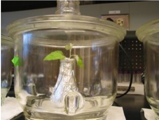
A 6-inch-tall experimental poplar cutting in a closed container absorbs and metabolizes gaseous benzene, a pollutant associated with petroleum. Credit: University of Washington
