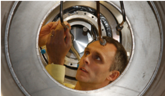
Philip Harris inspects the liquid helium supply pipes on the neutron Electric Dipole Moment cryostat
