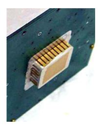
This sensor developed by Iowa State University researchers can detect leaks on spacecraft.
