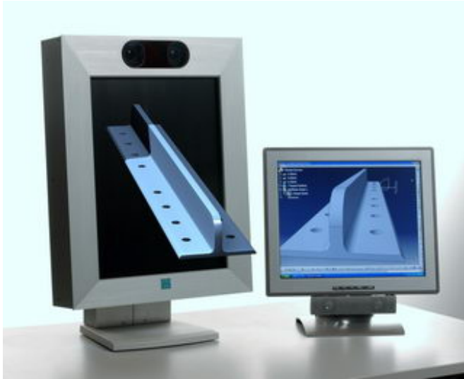
3D display shows the design engineer's projects and designs in 3D at the click of a button. © Fraunhofer HHI
