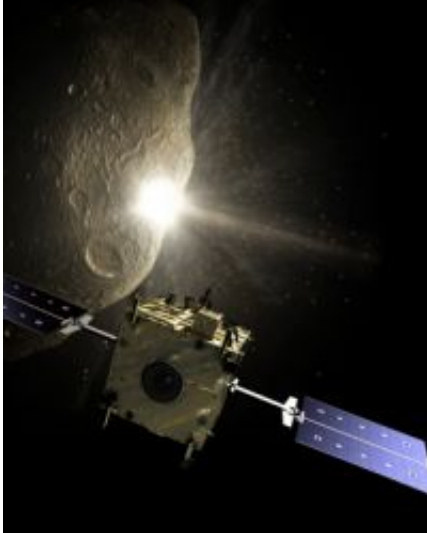
The key moment of the Don Quijote mission: the Impactor spacecraft (Hidalgo) smashes into the asteroid while observed, from a safe distance, by the Orbiter spacecraft (Sancho) Credits: ESA - AOES Medialab
