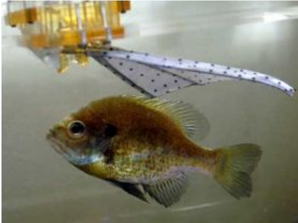
A bluegill sunfish swims in an MIT laboratory tank near a prototype of a robotic fin designed with the fish's fin as a guide. Photo / Donna Coveney
