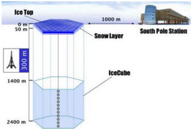
Diagram of IceCube. IceCube will occupy a volume of one cubic kilometer. Here we depict one of the 80 strings of optical modules (number and size not to scale). IceTop located at the surface, comprises an array of sensors to detect air showers. It will be used to calibrate IceCube and to conduct research on high-energy cosmic rays. Author: Steve Yunck, Credit: NSF
