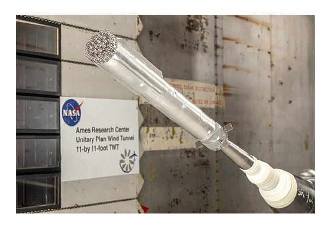
A 1.2% scale model of the Super Heavy rocket that will launch the Starship human landing system to the Moon for future crewed Artemis missions was recently tested at NASA's Ames Research Center's transonic wind tunnel, providing valuable information on vehicle stability when re-entering Earth's atmosphere. Credit: NASA
