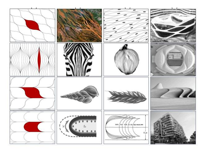
Examples of planar soft cells with two sharp corners in nature and in architecture. Left column: geometric soft cells. Middle columns: natural examples. Right column: examples from the architecture of Zaha Hadid. Credit: Wikimedia Commons, Google Earth, Krisztina Regős.
