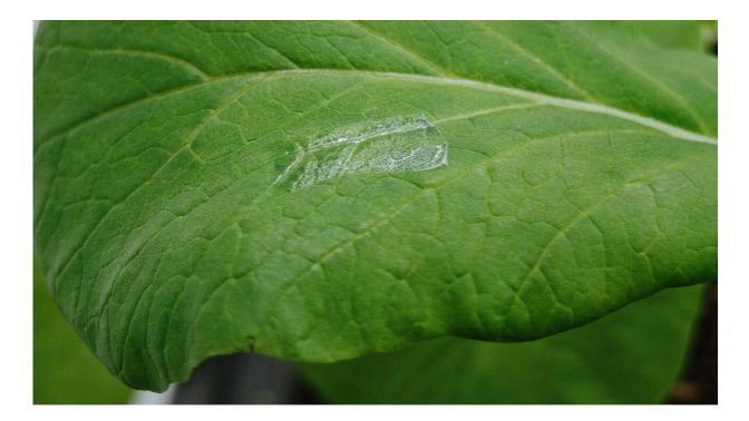
The innovative plant e-skin is ultrathin and transparent, allowing it to be seamlessly attached to the surface of plant leaves to collect data on key plant parameters, such as temperature and strain without hindering the plant's natural processes or causing physical damage to the plant. Credit: National University of Singapore
