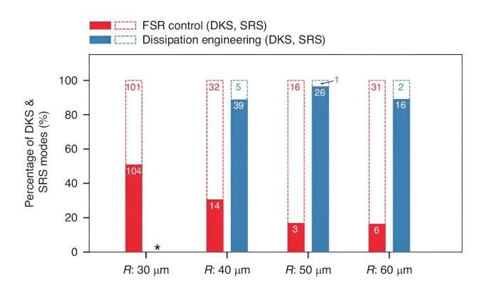
Percentage of microring modes that yield DKS states (solid) or SRS (dashed), utilizing the FSR control method (red) and dissipation engineering method (blue). Dissipation-engineered microrings with radius 30 µm were not attempted (star). A total of 396 modes across 94 microrings have been tested, where all microrings selected approximately satisfied design guidelines. Credit: *Light: Science & Applications* (2024). DOI: 10.1038/s41377-024-01546-7
