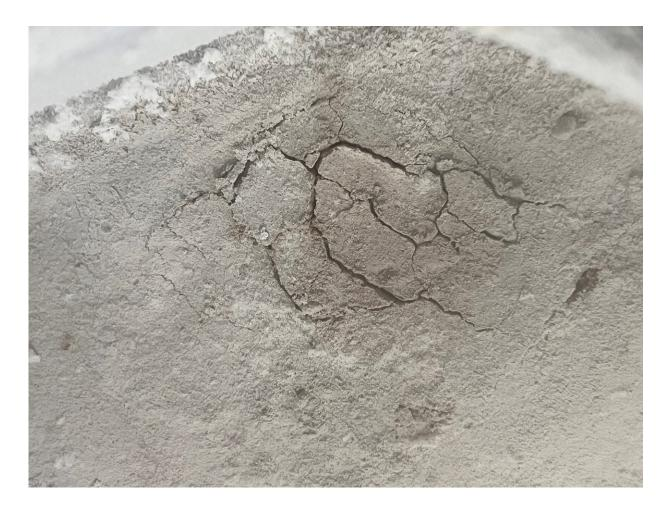
These formations similar to the Red Planet's "spiders" appeared within Martian soil simulant during experiments in JPL's DUSTIE chamber. Carbon dioxide ice frozen within the simulant was warmed by a heater below, turning it back into gas that eventually cracked through the frozen top layer and formed a plume. Credit: NASA / JPL-Caltech
