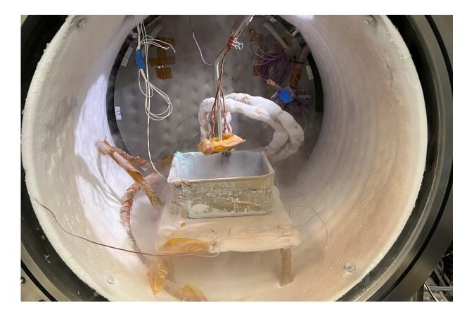
Here's a look inside of JPL's DUSTIE, a wine barrel-size chamber used to simulate the temperatures and air pressure of other planets – in this case, the carbon dioxide ice found on Mars' south pole. Experiments conducted in the chamber confirmed how Martian formations known as "spiders" are created. Credit: NASA / JPL-Caltech
