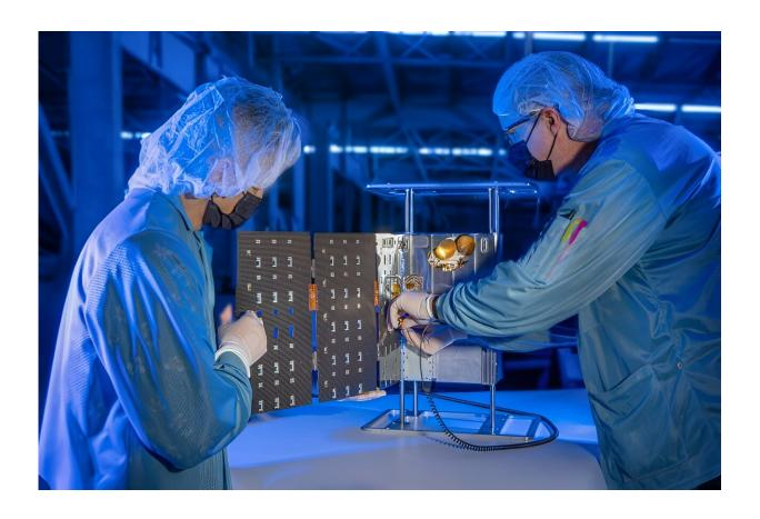
Technicians attach a solar array to one of the Electrojet Zeeman Imaging Explorer (EZIE) CubeSats. Credit: Brooks Freehill, Blue Canyon Technologies
