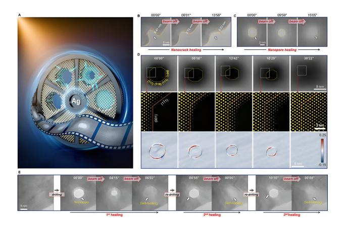
(A) An artistic poster depicting the autonomous self-healing phenomenon found in nanoscale Ag. (B, C) Sequential high-resolution TEM images showing the autonomous self-healing processes of a nanocrack (B) and nanopore (C) damage, respectively. (D) High-angle annular dark field (HAADF) images and the corresponding geometric phase analysis (GPA) of an overall self-healing process of nanopore. (E) Three runs of repeated reversible forming/healing cycles over the same region. Credit: IOP
