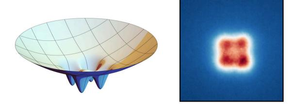
By creating indents on the reflective surfaces (shown on the left in an exaggerated form; the reflective surface is facing upwards), the researchers were able to imprint a structure onto the photon condensate (right). Credit: IAP / University of Bonn
