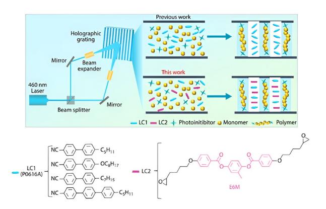
Schematic illustration on the construction of high-performance LC-based holographic polymer nanocomposites by doping E6M. P0616A was commercially available LC in nematic phase. Credit: *Chinese Journal of Polymer Science* (2024). DOI: 10.1007/s10118-024-3110-z
