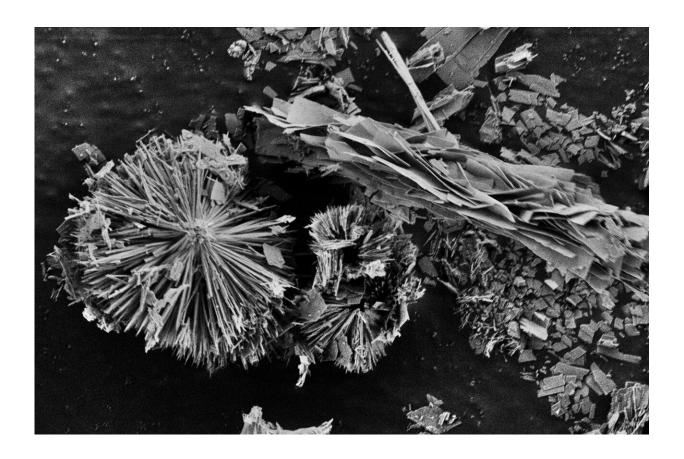
The surface of a Vanadium carbide MXene has been examined by Scanning Electron Microscopy. The beautiful structures are built by cobalt copper hydroxide molecules. Credit: B. Schmiedecke/HZB
