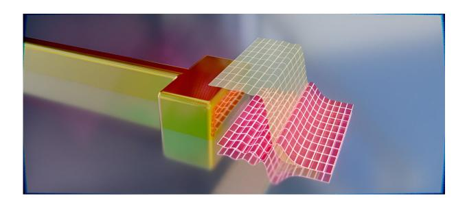
Artist's impression of an electrically contacted optical antenna (left) and the quantum mechanical distribution of its surface electrons. The normal distribution is shown in yellow, while the change induced by an applied voltage is shown in red. Credit: Thorsten Feichtner / Universität Würzburg
