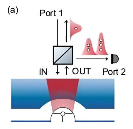
A schematic of a device to sift photons, showing a quantum dot surrounded by an optical cavity with a polarizing beam splitter above. Credit: Natasha Tomm et al, University of Basel and Ruhr University Bochumvia via CC-BY (4.0 International) license
