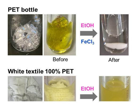
Before and after reactions of PET samples (top) and textile samples (bottom) with ethanol in the presence of FeCl<sub>3</sub>. Credit: Tokyo Metropolitan University
