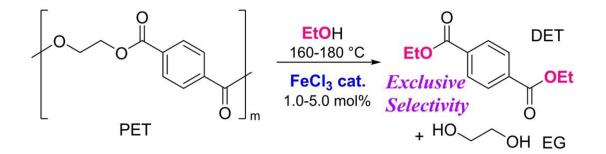
Acid-, base-free catalytic depolymerization of PET with ethanol by FeCl<sub>3</sub> catalyst. Credit: Tokyo Metropolitan University
