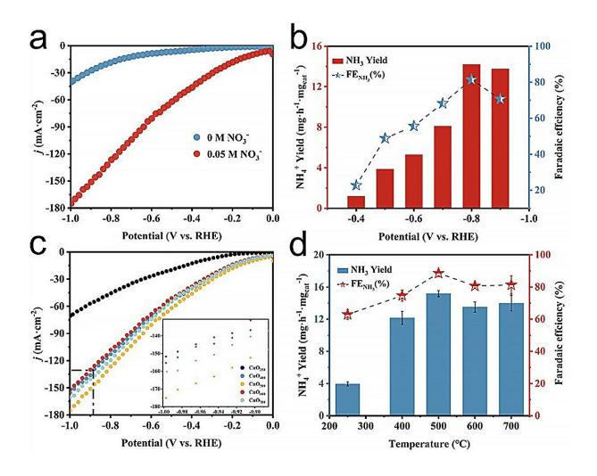
(a) LSV curves with and without  $NO_3^-$ . (b) Ammonia yield and FE after 2 h *i-t* electrolysis of  $CuO_{500}$ . (c) LSV curves of  $CuO_{250}$  (black),  $CuO_{400}$  (blue),  $CuO_{500}$  (yellow),  $CuO_{600}$  (red), and  $CuO_{700}$  (blue-green). (d) Ammonia yield and FE at -0.80 V after 1 h *i-t* electrolysis of the material with different calcination temperatures. Credit: *Advanced Science* (2024). DOI: 10.1002/advs.202404194
