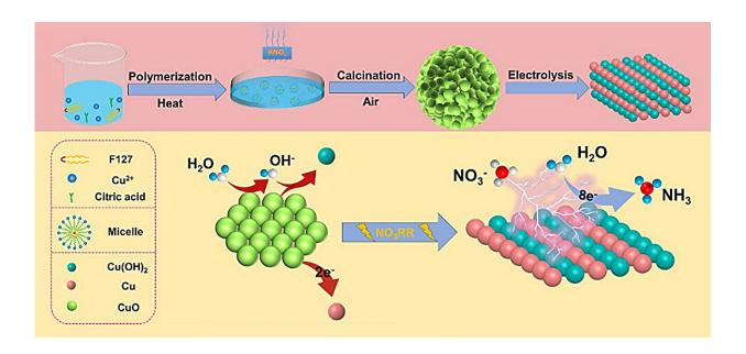
The CuO synthesis route and its reaction process at the cathode. Credit: *Advanced Science* (2024). DOI: 10.1002/advs.202404194
