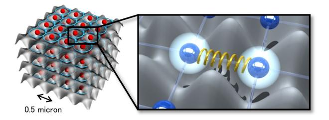
Atoms in the optical lattice, trapped at a distance of 0.5 micron, are excited to the Rydberg state by the ultrafast excitation technique. Interaction between close Rydberg atoms results in the repulsive force. Credit: Takafumi Tomita (Kenji Ohmori group)
