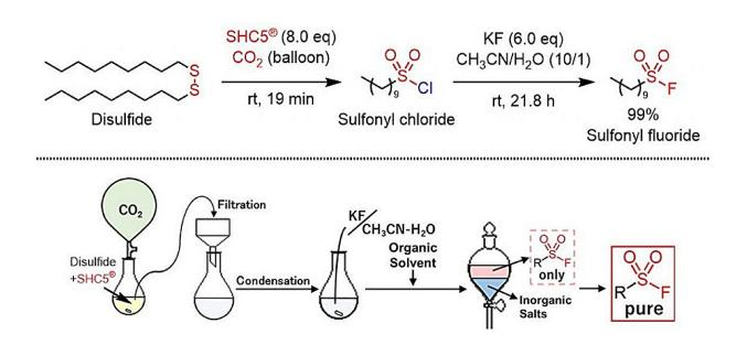
Low-cost synthetic reaction process for sulfonyl fluorides. Credit: *ACS Sustainable Chemistry & Engineering* (2024). DOI: 10.1021/acssuschemeng.4c03951
