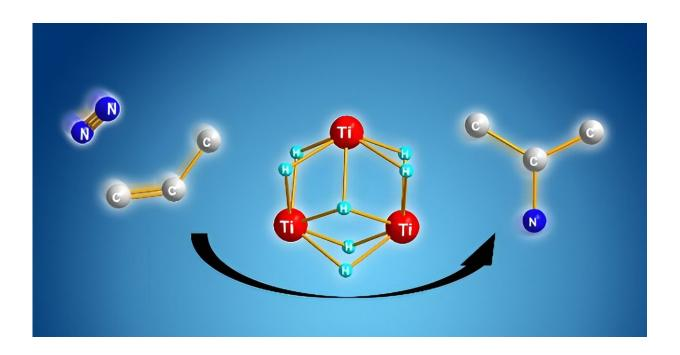
Titanium polyhydride (center) directly converts dinitrogen and a simple alkene (left) into an alkyl amine (right). Credit: Takanori Shima
