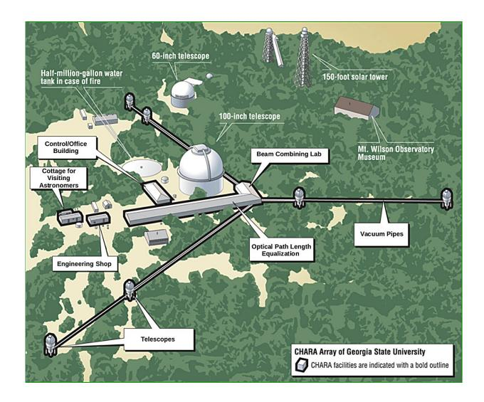
The CHARA Array is located at the Mount Wilson Observatory in the San Gabriel Mountains of southern California. The six telescopes of the CHARA Array are arranged along three arms. The light from each telescope is transported through vacuum pipes to the central beam combining lab. All the beams converge on the MIRC-X camera in the lab. Credit: Georgia State University
