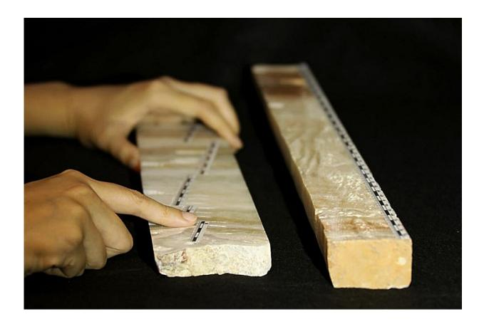
Limestone core samples collected Bàsura cave, northern Italy. The black-andwhite alternating bands represent a scale measured in centimeters. Researchers follow the scale to extract small subsamples ranging from 0.1 to 100 milligrams for carbon and oxygen isotope analysis, trace element determination, and uranium-thorium dating. Credit: National Taiwan University
