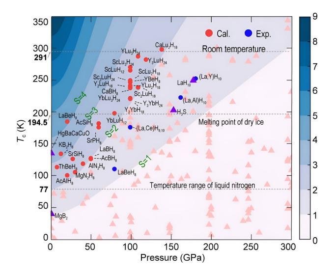
The relationship between superconducting transition temperature and pressure of ternary superconducting hydrides. The parabolic background represents the superconducting quality factor. Credit: Science China Press
