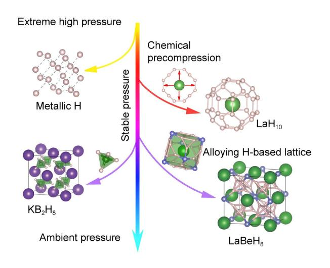
Pressure dependence of metallic hydrogen and hydride structures. Credit: Science China Press
