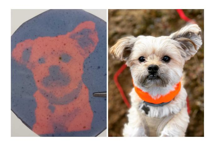
A two-dimensional light engraving (left) suspended in a polymer film. The original photo (right) was projected into the film using a red- and blue-light projector that activates a photosensitive additive in the polymer. Applying heat to the film will erase the image and make it ready to use again. Credit: Ivan Aprahamian/Sara Patch
