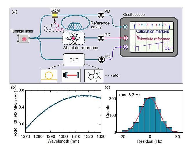
Principle of a Hz-level broadband spectrometer based on dual RF modulation. (a) Measurement scheme. A tunable CW laser is modulated by two RF signals  $(f_{mod1}, f_{mod2})$  via an electro-optic modulator (EOM). The modulated light is used
