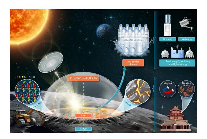
The strategy for in situ water production on the moon through the reaction between lunar regolith and endogenous hydrogen. Credit: NIMTE
