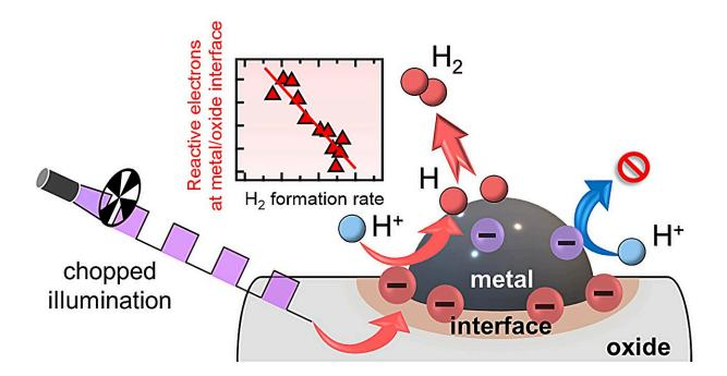
Schematic illustration of how the ST electrons contribute to photocatalytic  $H_2$
