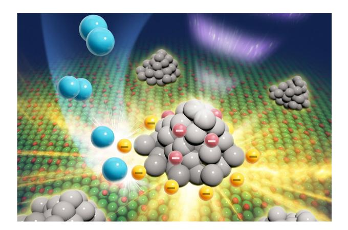
Schematic illustration of how the photogenerated electrons contribute to photocatalytic H<sub>2</sub> evolution reaction on metal-loaded oxides. Not the free electrons in metal cocatalysts but the electrons trapped in the periphery of cocatalysts directly contribute to the photocatalysis. This discovery was achieved by synchronizing periodic excitations of photocatalysts with a Michelson interferometer on *operando* FT–IR spectroscopy. Credit: Shinichiro Kinoshita
