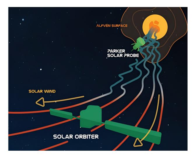
NASA's Parker Solar Probe and ESA's Solar Orbiter missions measured the same stream of plasma flowing away from the Sun at different distances. Parker measured lots of magnetic waves near the edge of the corona – called the Alfvén surface – while Solar Orbiter, located past the orbit of Venus, observed that the waves had disappeared and that their energy had been used to heat and accelerate the plasma. Credit: Arya De Francesco
