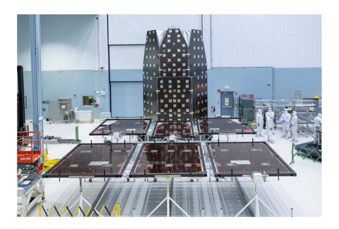
Both versions of the Solar Array Sun Shield for NASA's Nancy Grace Roman Space Telescope appear in this photo, taken in the largest clean room at NASA's Goddard Space Flight Center. The flight version lies flat in the foreground, while the qualification assembly stands upright in the background. The flight panels will shade the mission's instruments and power the observatory. Credit: NASA/Chris Gunn
