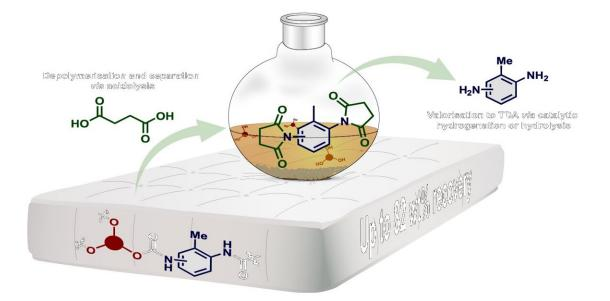
The graphic shows how the new combination of acidolysis and hydrolysis can recover up to 82 weight percent of the original material from flexible PUR foam—used in mattresses—as two separate fractions of diamines and polyols. The diamine is shown as TDA (toluene diamine). Credit: Thomas Balle Bech, Aarhus University
