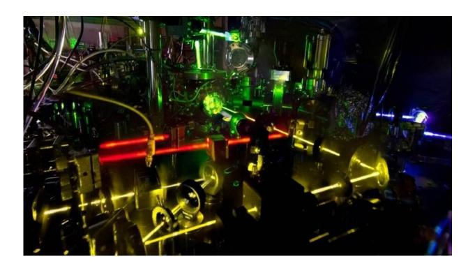
A Ytterbium optical lattice clock setup with the associated optics and vacuum setups. Credit: Andrew Ludlow @ NIST
