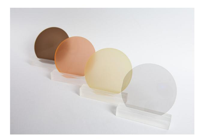
The different color nuances of the AlYN/GaN wafers result from different yttrium concentrations and growth conditions. Credit: Fraunhofer IAF
