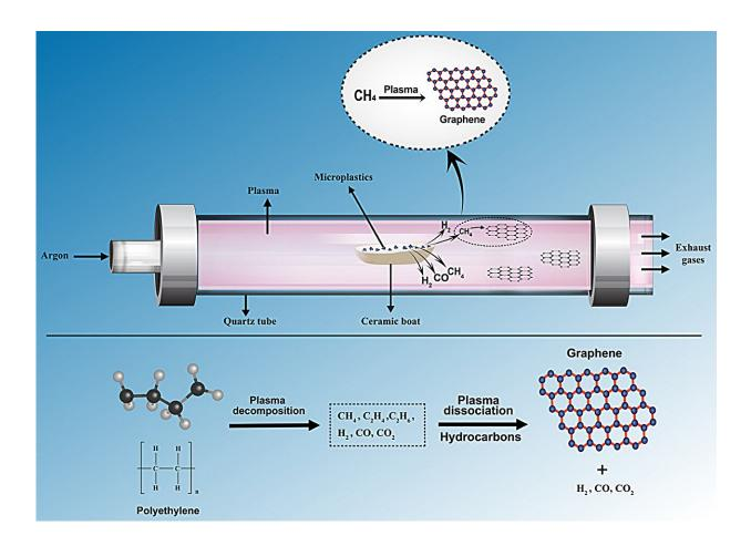
Schematic representation of APMP system for the synthesis of graphene from PE microplastics. Credit: From *Small Science* (2024). DOI: 10.1002/smsc.202400176
