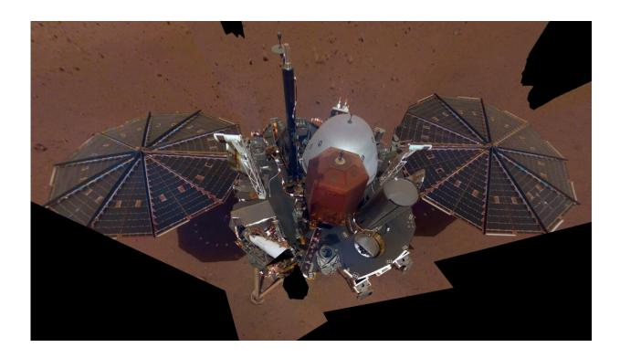
NASA InSight's first full selfie on Mars. It displays the lander's solar panels and deck. On top of the deck are its science instruments, weather sensor booms and UHF antenna. The selfie was taken on Dec. 6, 2018 (sol 10). The selfie is made up of 11 images which were taken by its Instrument Deployment Camera, located on the elbow of its robotic arm. Those images are then stitched together into a mosaic. Credit: NASA/JPL-Caltech
