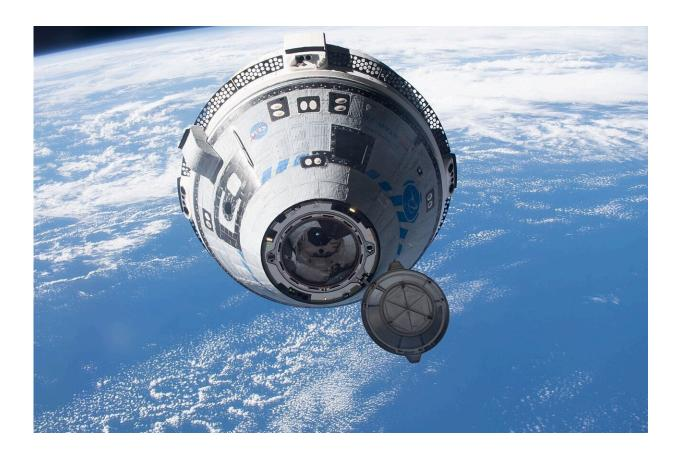
Boeing's CST-100 Starliner crew ship approaches the International Space Station on the company's Orbital Flight Test-2 mission before automatically docking to the Harmony module's forward port. The orbiting lab was flying 268 miles above the south Pacific at the time of this photograph. Credit: Bob Hines/NASA
