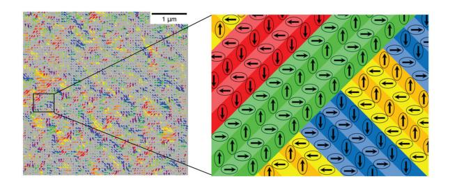
The image on the right shows the alignments of dipole directions in mesoscale structures within region of the relaxor ferroeletric material shown in the left image. Credit: Argonne National Laboratory.
