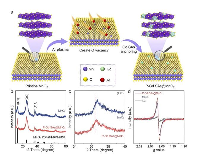
(a) The schematic route for the synthesis of P-Gd SAs@MnO<sub>2</sub> nanosheets; (b, c) XRD patterns of P-Gd SAs@MnO<sub>2</sub> and MnO<sub>2</sub>; (d) EPR spectrum of P-Gd SAs@MnO<sub>2</sub>, MnO<sub>2</sub>, and blank CC. Credit: Hao Li et al.
