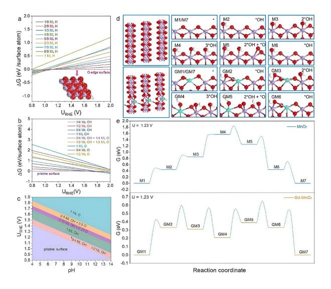
Surface Pourbaix diagrams: (a) H coverage for  $MnO_2$  slice with  $Mn_6c-O_3c$  chain, (b) oxygen species coverage for  $MnO_2$  slab with  $Mn_5c$  and  $O_2c$  sites. (c) 2D surface Pourbaix diagram showing URHE vs. pH. (d) Geometric structures of  $MnO_2$  and Gd- $MnO_2$  with various oxygen intermediates. (e) OER free energy diagrams for  $MnO_2$  and Gd- $MnO_2$  at 1.23 V. Pink, green, red, and white spheres denote Mn, Gd, O, and H, respectively. Credit: Hao Li et al.
