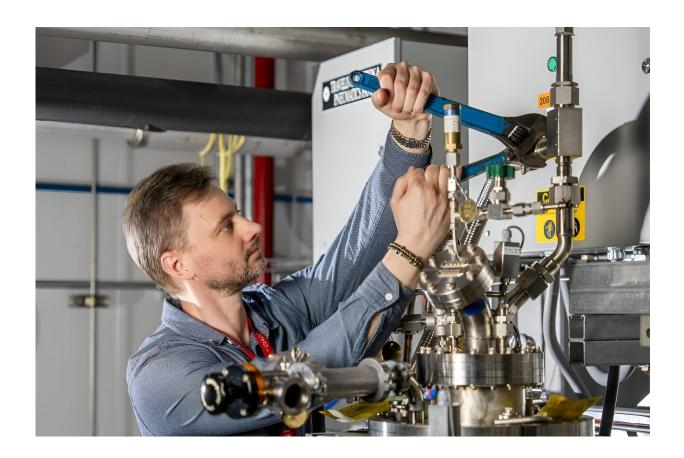
Fermilab engineer Sergey Koshelev works on equipment that regenerates the filters used for purifying liquid argon. Credit: Dan Svoboda, Fermilab
