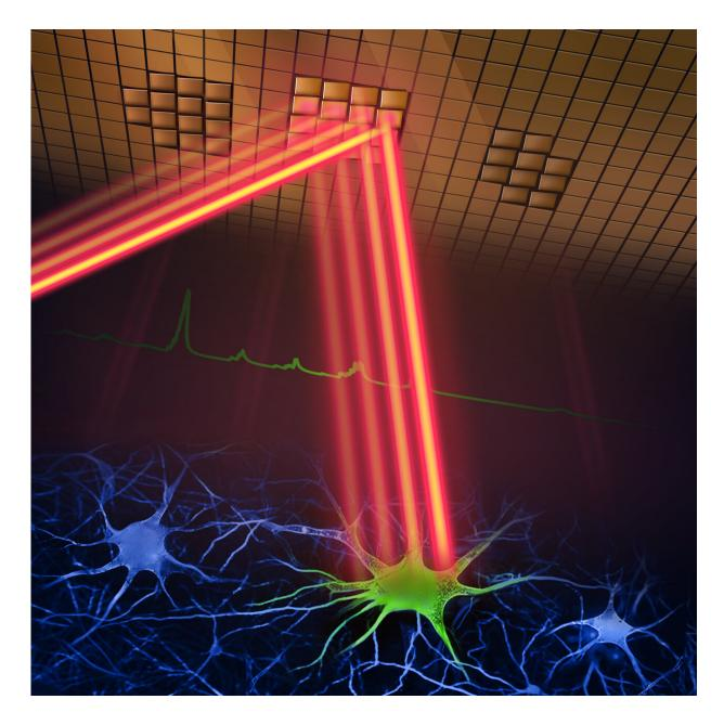
A new two-photon fluorescence microscope can capture high-speed images of neural activity at cellular resolution thanks to a new adaptive sampling scheme and line illumination. The illustration shows the adaptive sampling scheme, in which a laser beam patterned by a digital micromirror device selectively illuminates neurons in the brain tissue to image their activity. Credit: Wei Wei and Mei Xueting, LINGO.AI LLC
