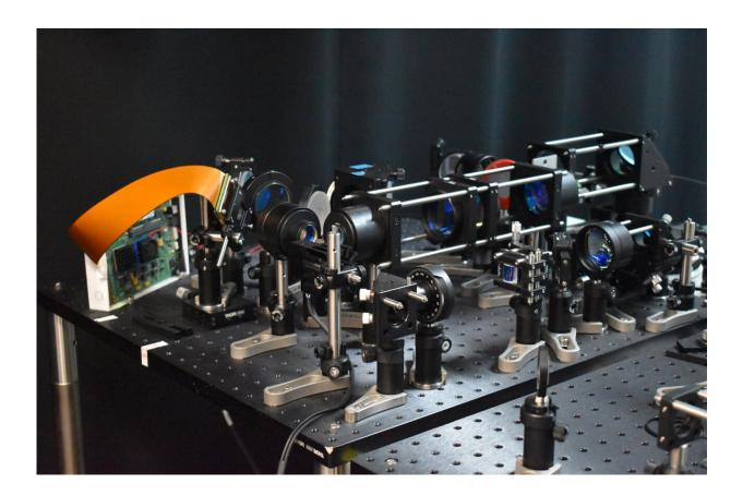
The experimental setup shows the optical components, including the DMD and beam scanners, for the two-photon microscope with the adaptive line-excitation scheme. Credit: Molly M Bechtel, University of California, Davis
