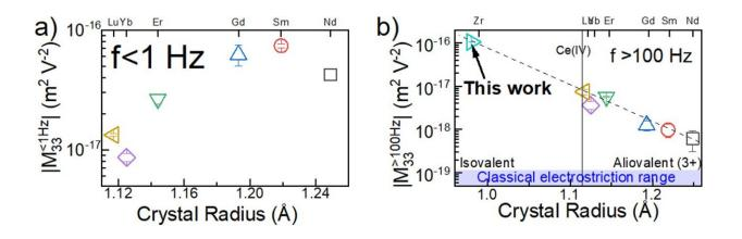
Longitudinal electrostriction strain coefficient of 10 mol% doped ceria ceramics as a function of dopant crystal radius. Credit: *Nature Communications* (2023). DOI: 10.1038/s41467-023-43032-5
