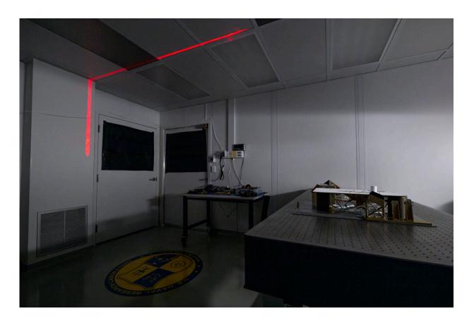
The Light-sheet Anomaly Resolution and Debris Observation (LARADO) instrument undergoes alignment verification in Washington, D.C., July 2, 2024. The LARADO instrument will create a fan of light through a dispersive optic to detect debris in space and increase the safety of manned and unmanned spacecraft. Credit: U.S. Navy / Sarah Peterson)
