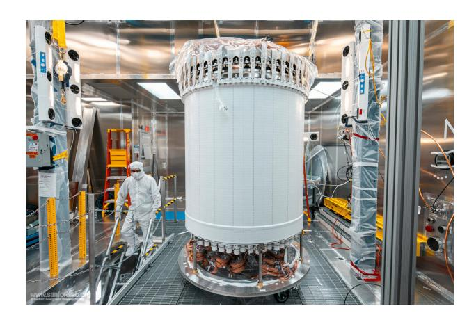
LZ's central detector, the time projection chamber, in a surface lab clean room before delivery underground. Credit: Matthew Kapust/Sanford Underground Research Facility
