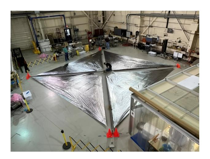
The ACS3 being unfurled at NASA's Langley Research Center. The solar wind is reliable but not very powerful. It requires a large sail area to power a spacecraft effectively. The ACS2 is about 9 meters (30 ft) per side, requiring a strong, lightweight boom system. Credit: NASA
